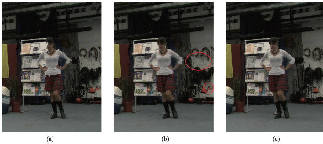
Figure 8 Illustration of the role of segmentation and view-interpolation→multi-view reconstruction→view interpolation pipeline. (a) Result without image segmentation procedure; (b) Result without optimization from reconstruction; (c) Result with optimization.
